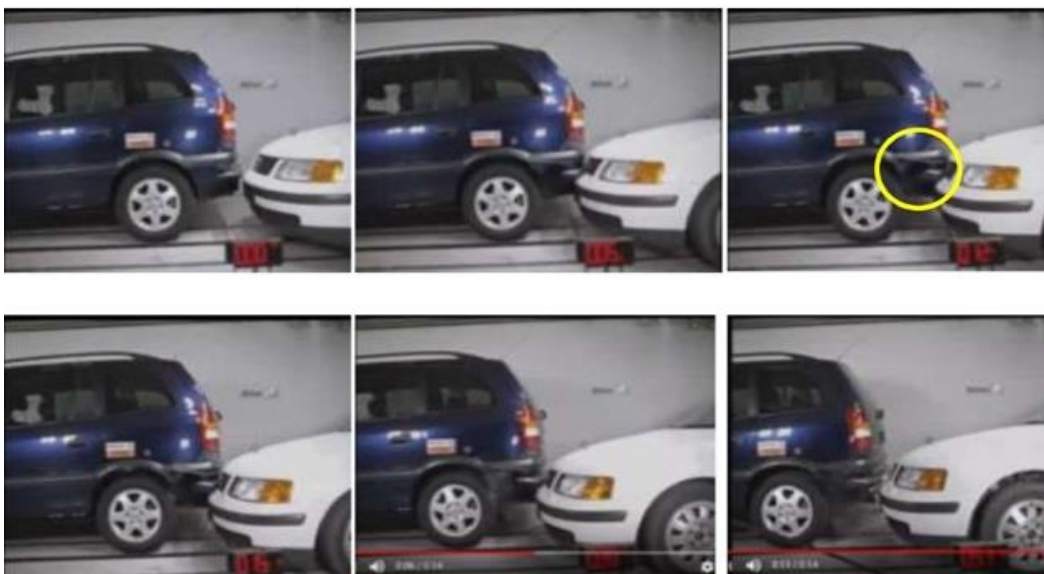
Fig.11 View Crash Test Sequence with Bumper Movement
