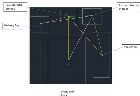
Fig 9 Alternative Space Relationship diagram with the finished product and raw material storage swapping locations
