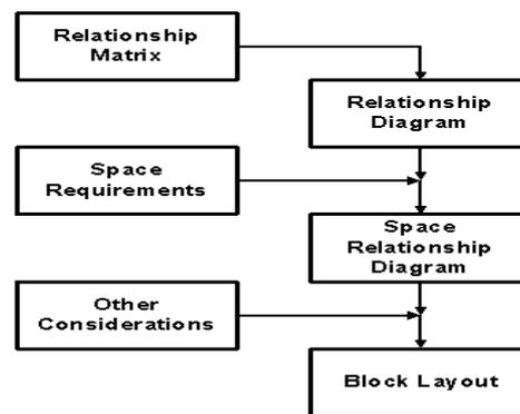
Fig 1. An illustration of the main outputs of the SLP procedure
