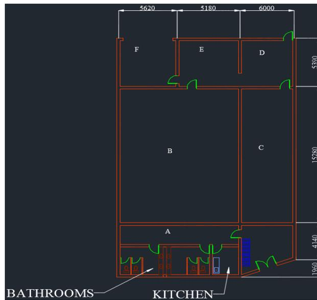
Fig 13 Suggested final layout and arrangement of the partitioning on the ground floor
