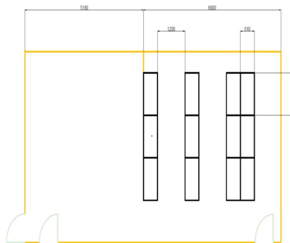
Fig 10 Recommended layout for the Finished Product storage section
