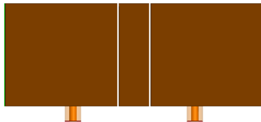
Fig. 10. 1x2 antenna with planer ladder shaped coplanar EBG
