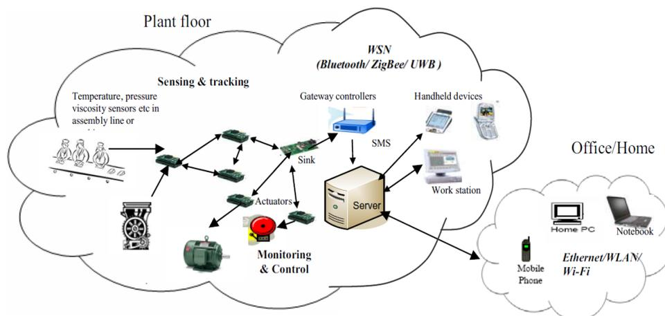
Figure 1. A typical industrial wireless sensor network [3].
